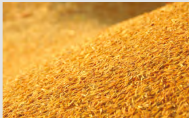
Paddy husk – an alternative fuel source to power the kiln.
