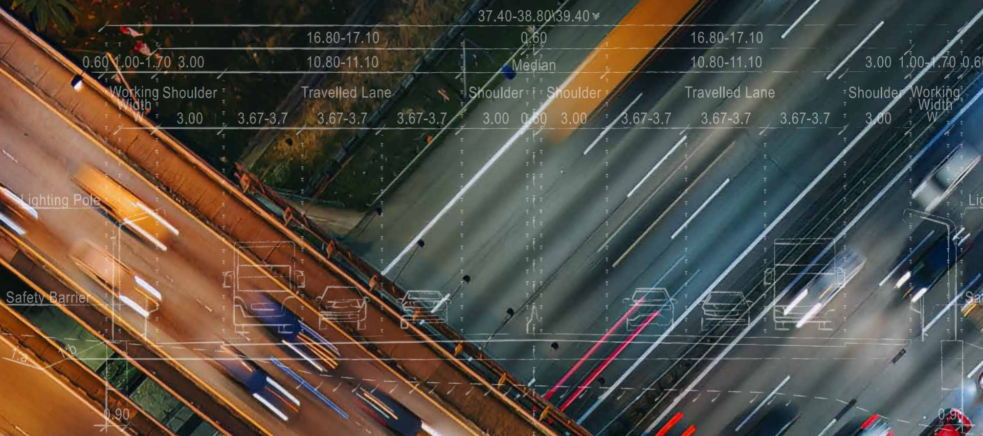
Fig.2 6-lane Expressway Cross Section
